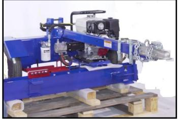
Install the tongue and reinstall the bolts and tighten.
