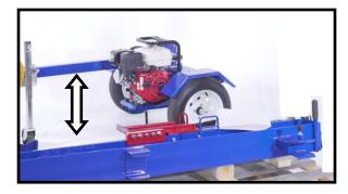
Using a fork lift or engine hoist, attach a sling to the end of the boom, raise the beam up to the upright position. If no lift is available it can be raised by three people. Have two people lift while the other stabilizes the base on the ground to prevent slipping out. On a level hard surface, the beam will stand upright and the base can be wheeled up to the upright beam.
