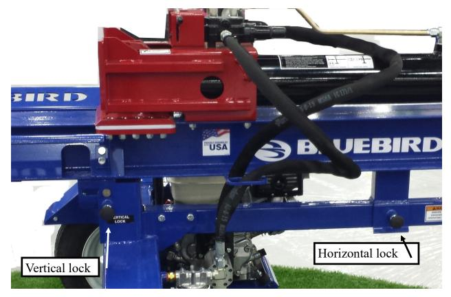
• The unit can be operated either horizontal or vertical. There is a pin which locks the unit in either position. To use vertically, release the horizontal pin and tilt unit upright and lock into place with the vertical pin. To return the unit horizontally, release the vertical pin and tilt the unit back to the horizontal position, then lock it's pin in place. The knob will close completely when it is secured.
