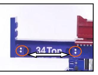
Remove the four bolts on each side and attach the side plates.
